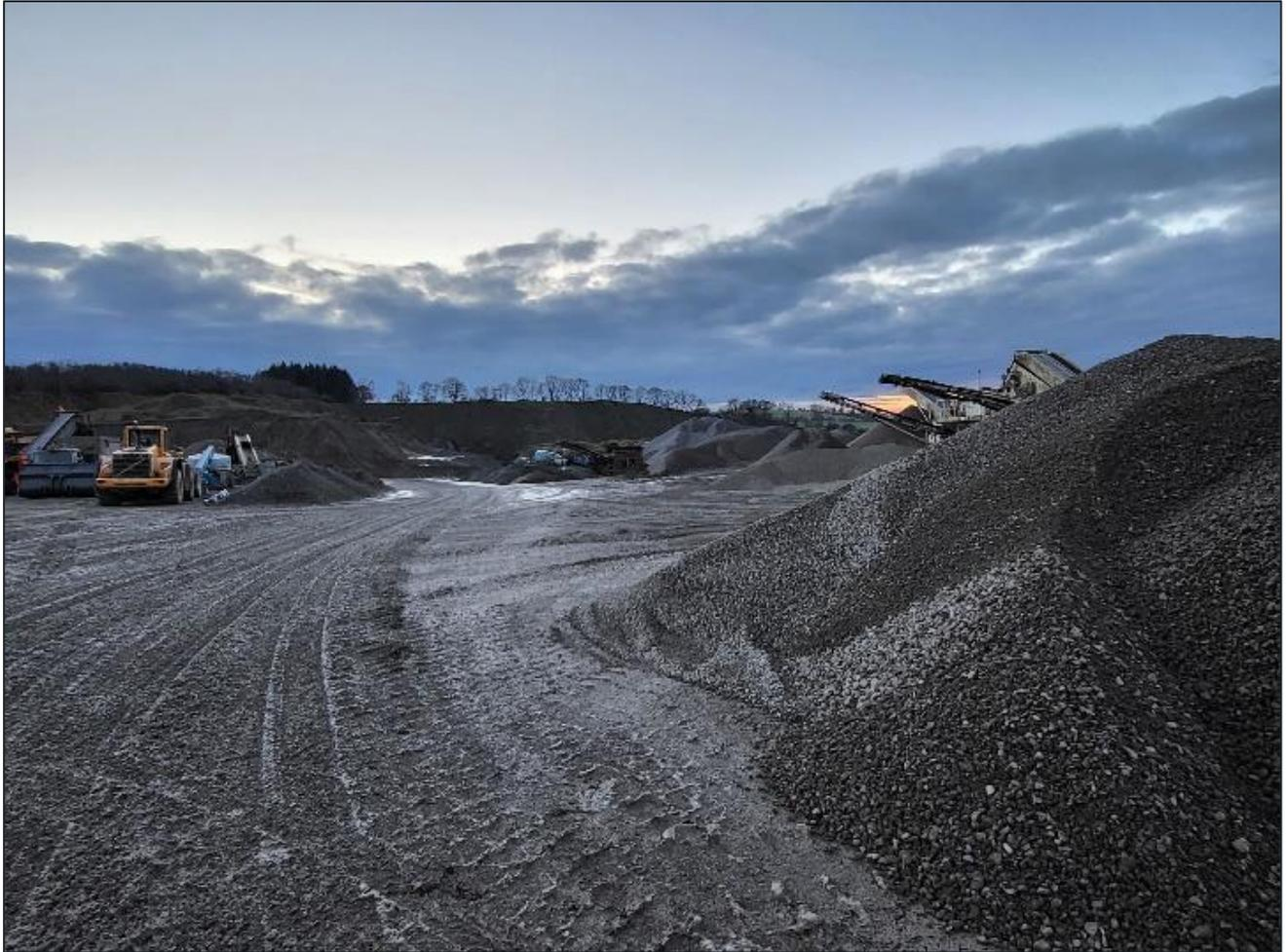
**Figure 11-15: Current temporary stockpiling off of the extracted material next to the processing plant in southeastern end of the quarry**
